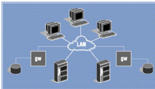
A NAS gateway provides the function of a conventional NAS appliance but without integrated disk storage. The disk storage is attached externally to the gateway, possibly sold separately, and may
