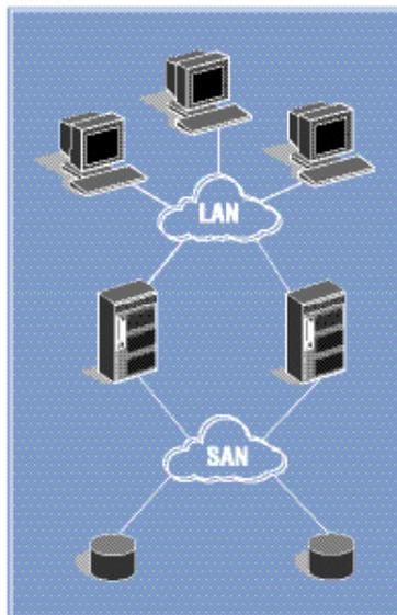
**SAN: Storage Area Network.** Storage resides on a dedicated network. Like DAS, I/O requests access devices directly. Today, most SANs use Fibre Channel media, providing an any-to-any connection for processors and storage on that network. Ethernet media using an I/O protocol called iSCSI is emerging in 2001.
