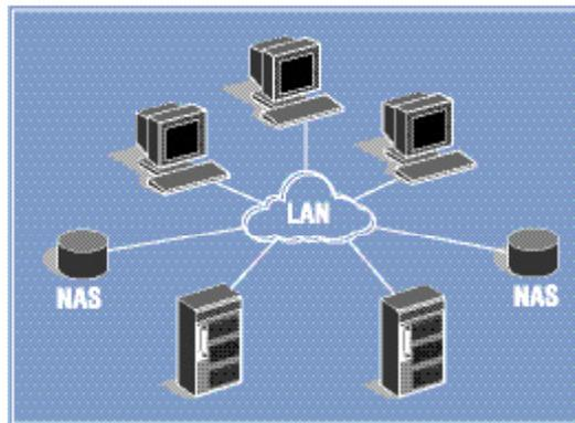
A NAS is a device that resides on a network that may be shared with non-storage traffic. Today, the network is usually an Ethernet LAN, but could be any network that supports the IP-based protocols that NAS uses.
