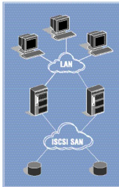
iSCSI is a proposed industry-standard that allows SCSI I/O commands to be sent over a network using the popular TCP/IP protocol. This is analogous to the way SCSI commands are already mapped to Fibre Channel, parallel SCSI, and SSA media. The proposal was made to the IETF (Internet Engineering Task Force) standards body jointly by Cisco Systems, Inc. and IBM, and is expected to be ratified in mid 2001. The iSCSI standard is also supported by SNIA (Storage Networking Industry Association).
